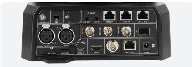
Equipped with HDMI, 12G-SDI, 3G-SDI, USB, and LAN interfaces, it can output 5 digital signals at the same time. It also supports camera control using RS232, RS422, network and USB. The device has strong compatibility and can be widely used in various scenarios.
